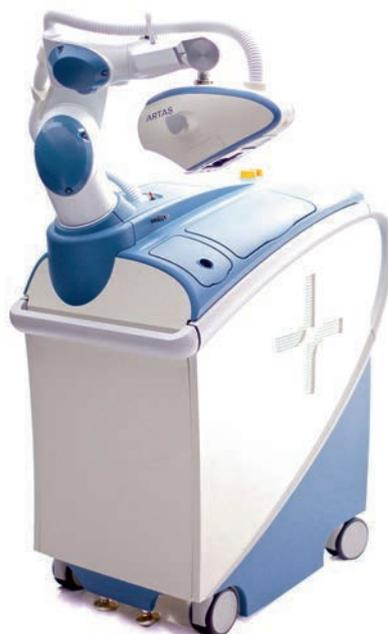
**The ARTAS Robotic System uses precision robotics to carry out FUE procedures**
